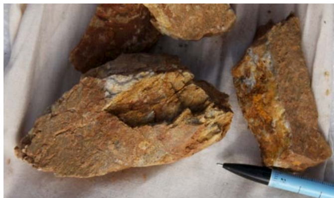
Picture 2 - Sample D033-1, 51.3gms/tonne Gold and 20.8gms/tonne Silver: Historic Mine Breccia Lode 3, Bangadang area. Sheared metasediment hosting sheeted quartz veins with yellow limonite staining after sulphides
