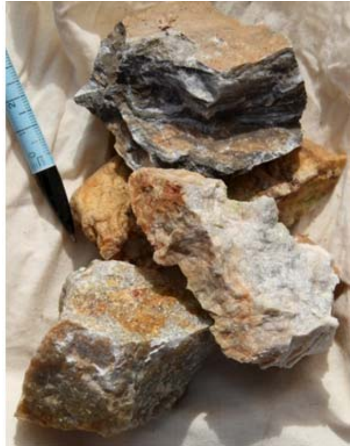
Picture 4 - Sample D025-1, 24.9gms/tonne Gold: Historic Mines Nacki Nacki Eluvial, Bangadang area. Float consisting of narrow quartz veining hosted in foliation of metasediments and fragments of quartz veins
