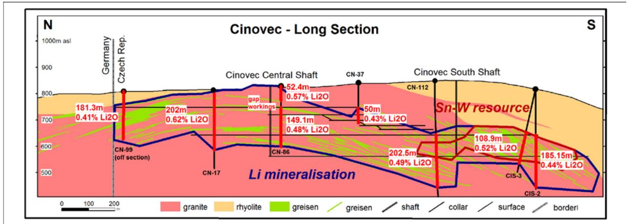
Figure 1 – Cinovec schematic long section showing select lithium drill intercepts
