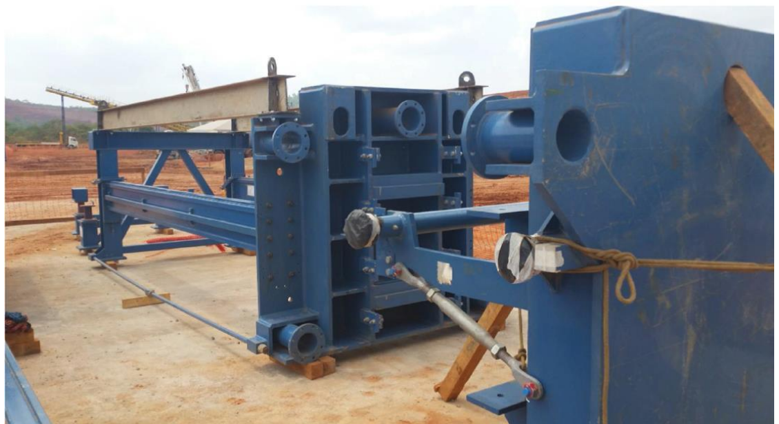
Metso VPA plate and frame pressure filter main assembly ready for installation within the building
