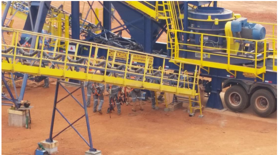
Secondary cone crusher/screen of local manufacture, being configured to produce a -20mm sized feed to the ball mill. The ball mill feed will be stockpiled above the reclaim tunnel below
