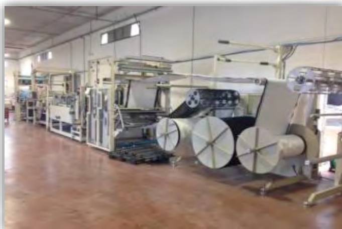
Picture #6 - SABRE membrane manufacturing machine in Emefcy's production facility
