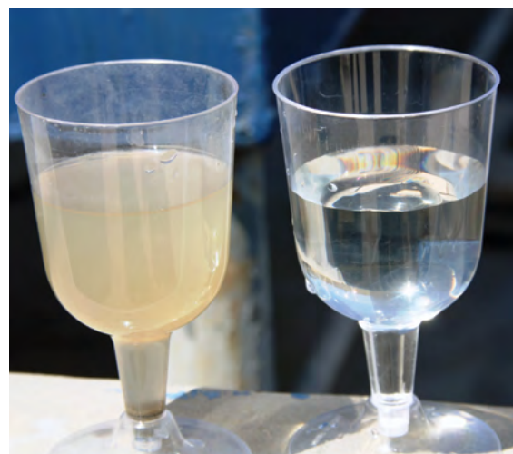
SABRE input and output water from demonstration plant.
