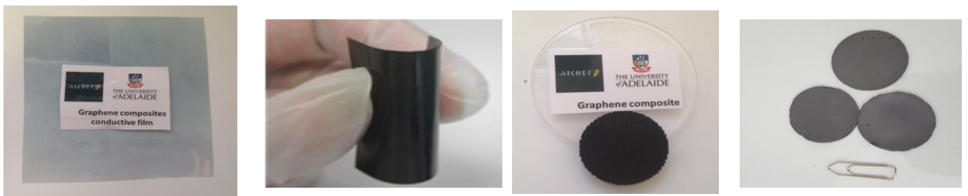
Figure 2. Selected graphene products produced from Archer graphite (graphene conductive film, conductive flexible polymer, graphene composite and electrodes for battery and supercapacitor applications)
