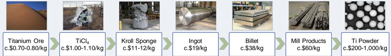
Metalysis technology simplifies and can dramatically reduce the cost of metal powder production
