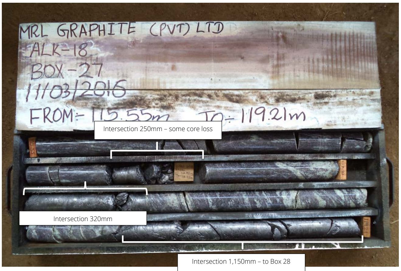
Figure 1: Core from drill hole ALK18- boxes 27
