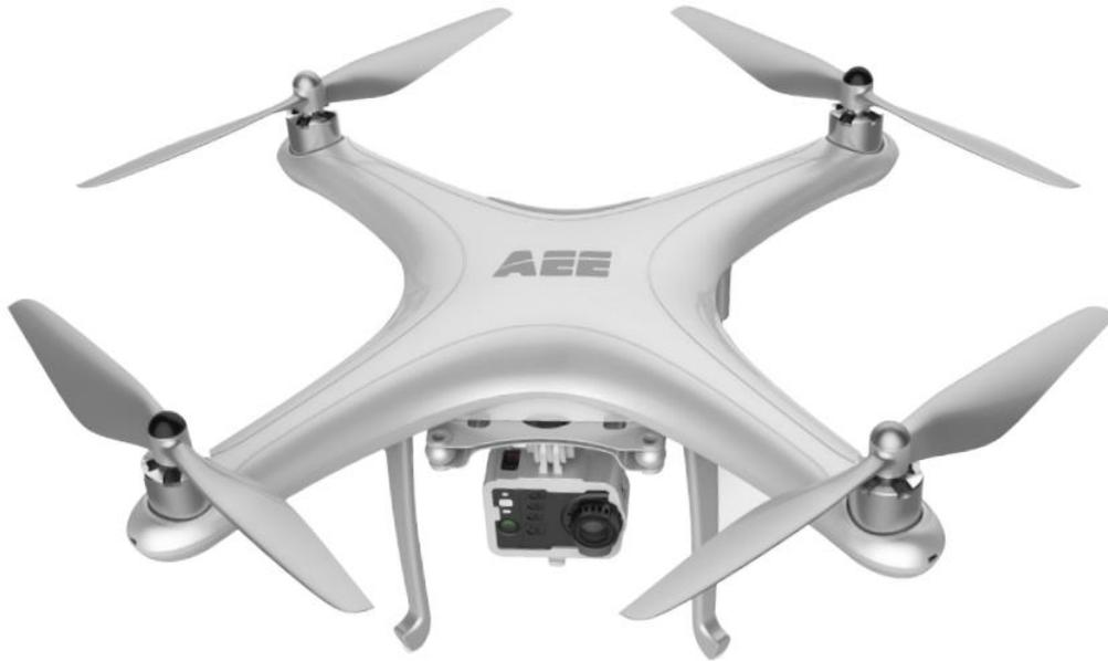
The **AEE Lyfe Silver Camera** comes with built-in Bluetooth and WiFi, is capable of 16 MP photo resolution and 4K video recording, and supports up to 64GB SD card.
