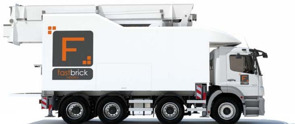
Figure 2 - The Hadrian X in its compact, "road-capable" form. Brick pallets are loaded into the back of the truck and robotically de-hacked and loaded onto the conveyor
