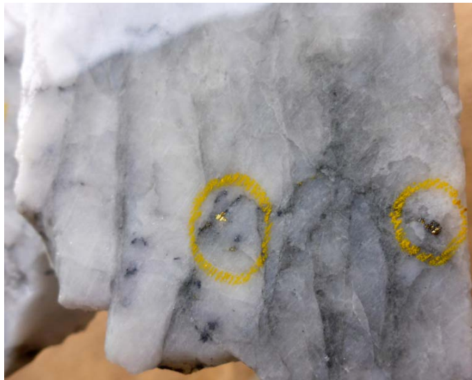
Visible, free milling gold in White Deer Reef, HQ Core 63.5mm in diameter.
