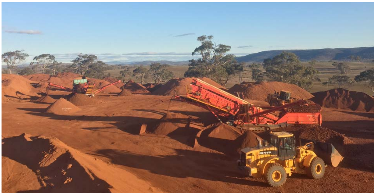
Figure 1: Screen operations at Bald Hill Bauxite Project in Spring 2015
