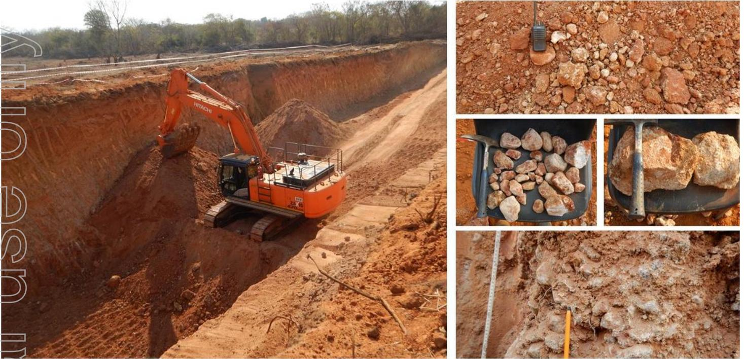
**Figure 3: Pit 21. (i.) Excavation of Pit 21 down to 8m; (ii.) Gravel layer in the stock pile; (iii.) Gravel clasts of quartzite ranging from 2cm to 8cm in diameter, (iv.) Angular quartzite clasts approximately 15 cm in diameter and (v.) Gravel layer red oxidised material with white nodules and clasts**
