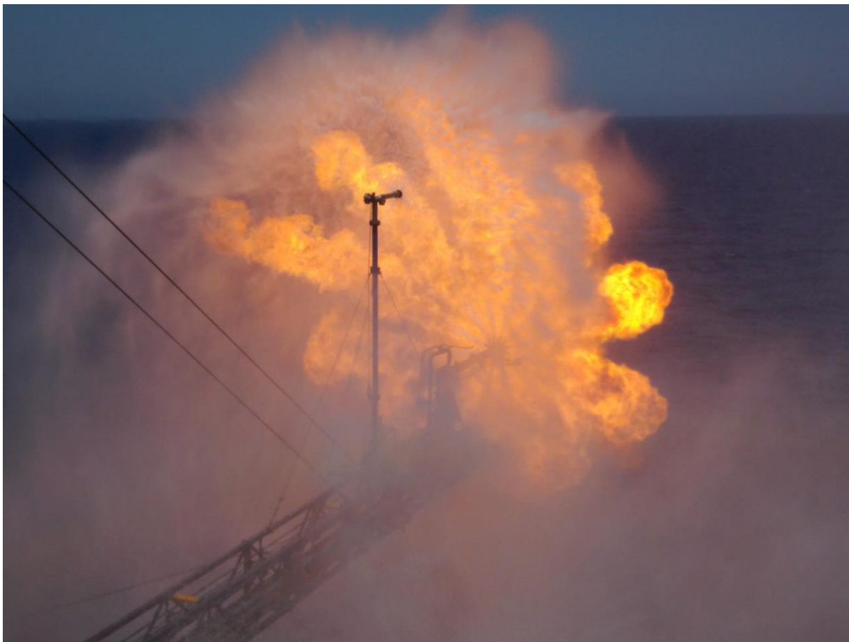
Annexure 1: Images of the Ocean Monarch undertaking flow test operations, with gas and condensate successfully being flowed to surface.
