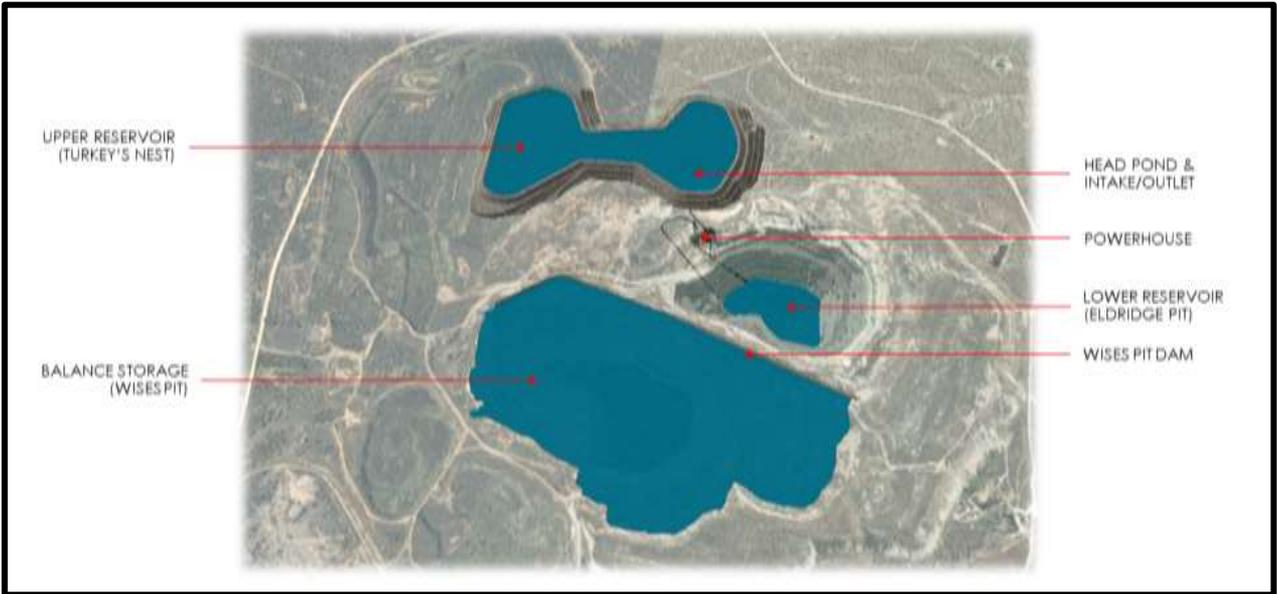
**Figure 1:** Aerial Pictorial Representation of the General Arrangement
