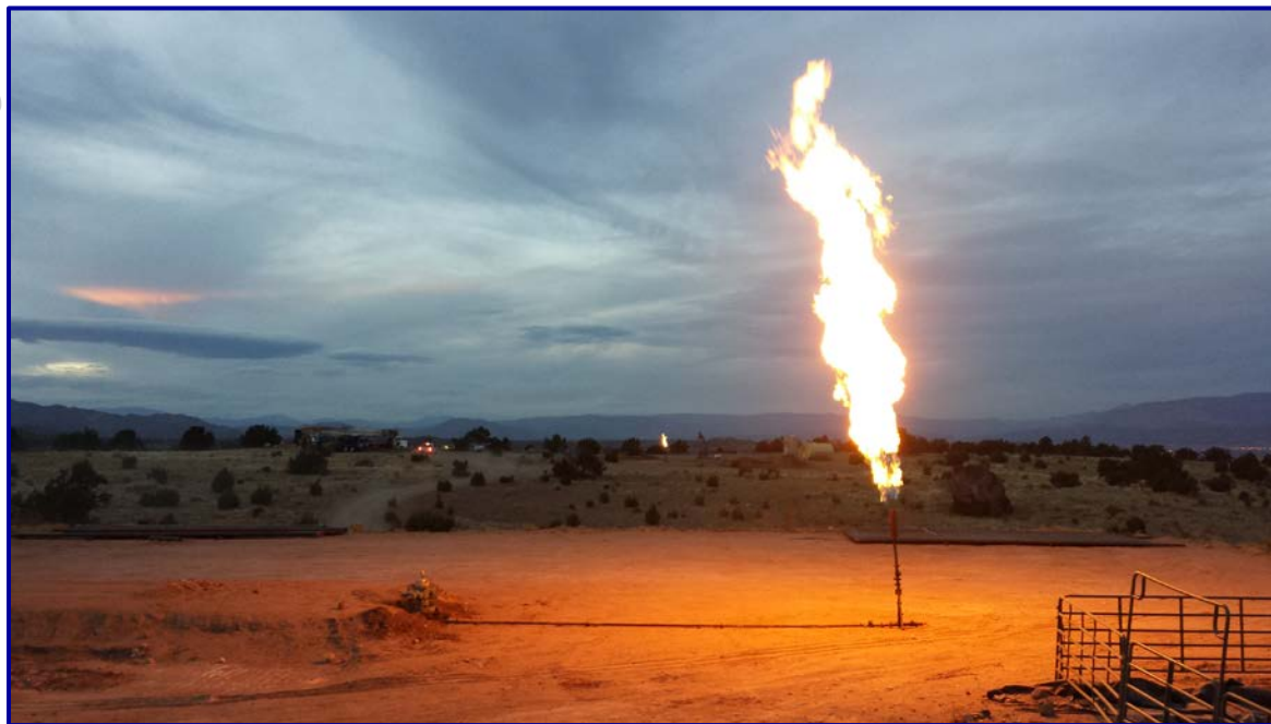
Marco Polo # 1 well – gas being flared ahead of flow tests for oil
