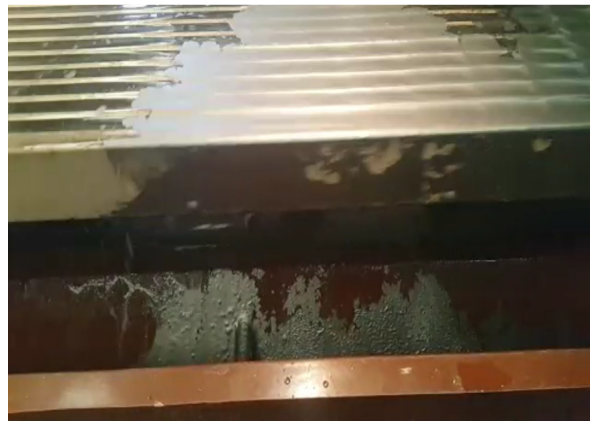
Figure 3 shows graphite from Namanagle that has gone through the crushing and flotation process and the final step to prepare it in a concentrate form.
