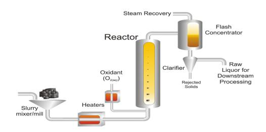
For lignite and lignin most the material is chemically converted [the OHD process] with a reaction time of less than a minute. The output from the reactor is a liquid which is about 98.5/99.5%% water, and 1.5/0.5% by weight organic chemicals in solution (the bio-stimulant fertiliser).
