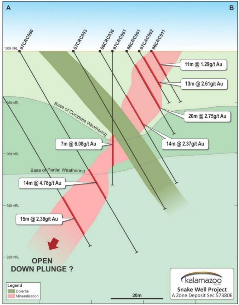
**Figure 3. Cross section A-B through A-Zone mineralisation**
