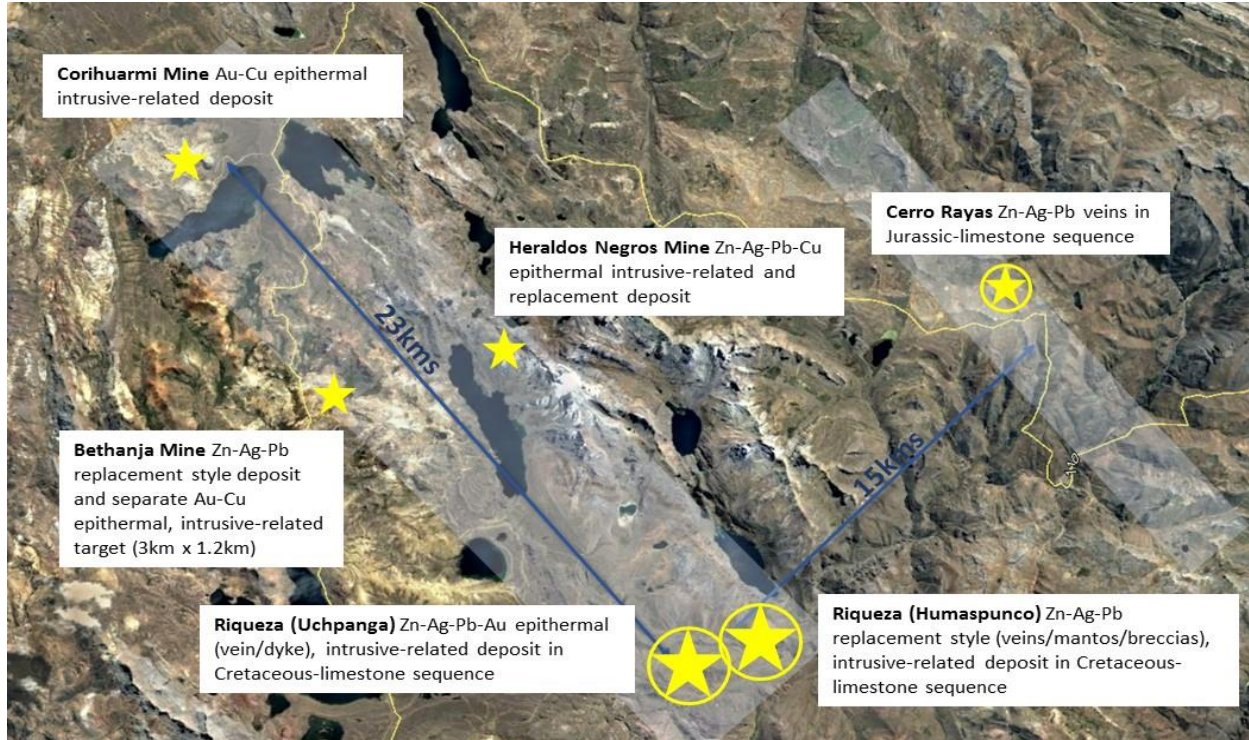
Figure 4: ABOVE A regional plan showing the location of Riqueza in relation to mines in the vicinity, the Corihuarmi Au-Cu Mine, the Bethanja Zn-Ag-Pb Mine, the Heraldos Negros Zn-Ag-Pb-Cu Mine. This important mineral belt, denoted by a broad pale blue line, runs parallel to regional mountain building processes such as compressional folding, thrusts and faults, and magmatic emplacements (stock intrusions). A parallel mineral belt hosts Cerro Rayas.
