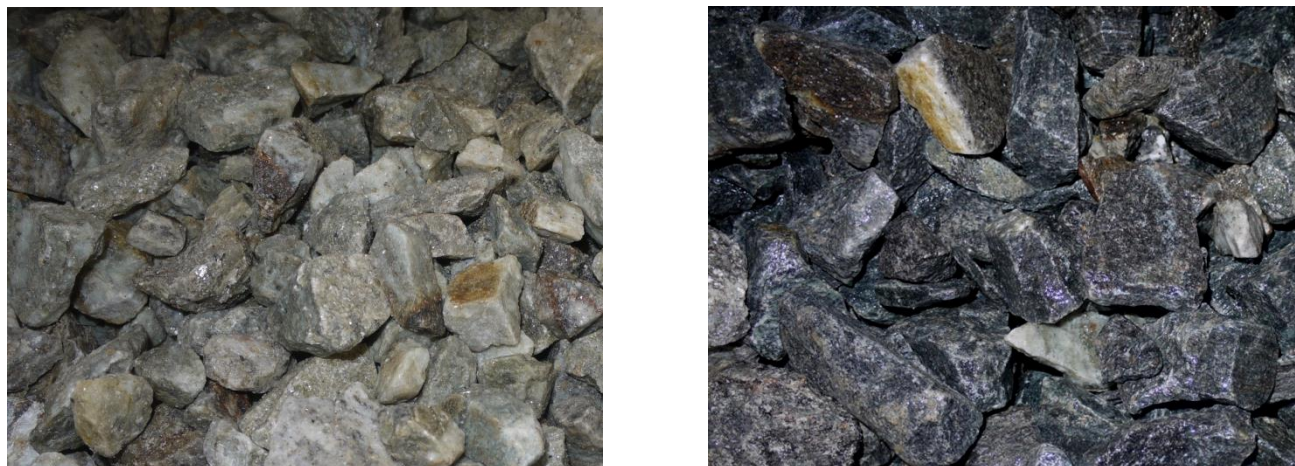
Figure 3: Sorting of -70 + 25 mm AHP. Lithium bearing pegmatite product (left) and amphibolite reject (right)
