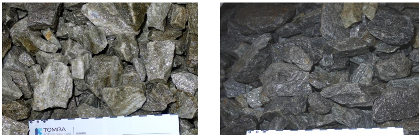
Figure 2: Sorting of -70 + 25 mm MHP. Lithium bearing pegmatite product (left) and mica schist reject (right).
