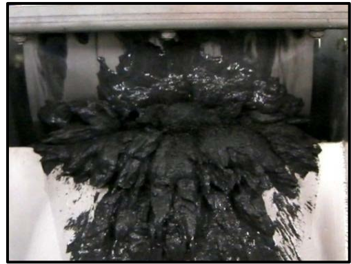
After second magnetic separation 66%Fe
