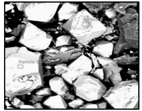
Elutriation removes free silica upgrade > 69%Fe
