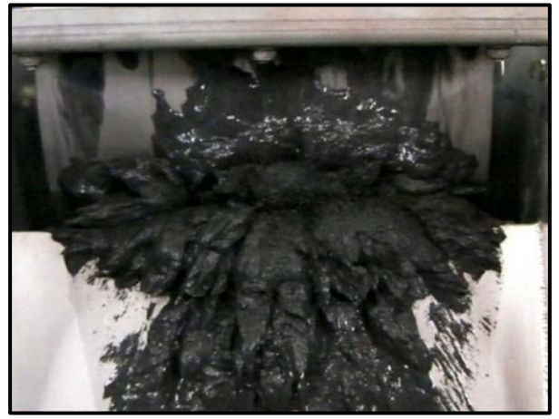
45% rejection at first magnetic separation
