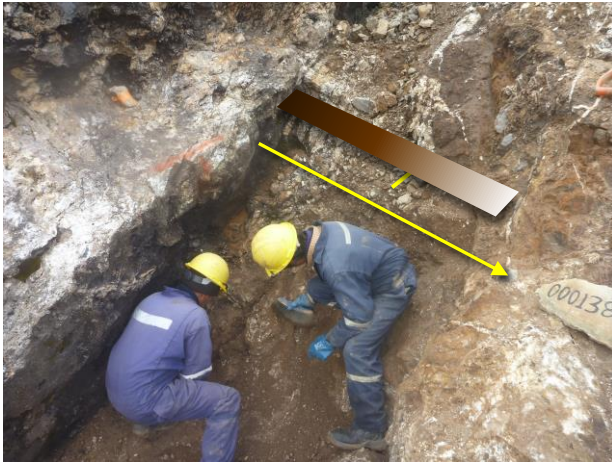
Figure 3 LEFT A large vein, over two metres wide, is being prepared for sampling. The sulphides that occur within the vein appear to concentrate towards the hanging wall (left hand margin). This is seen by the gradual increase in brown colouring (oxidised and semi-gossanous sulphides) to the left across the vein. The vein also hosts large masses and veins of barite (cream colouring).
