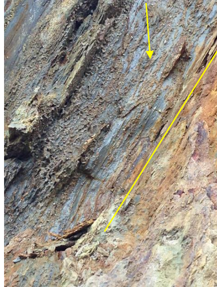
Image 3: Close-up of near pure Zinc mineralisation exposed in wall of Gibson’ pit.
