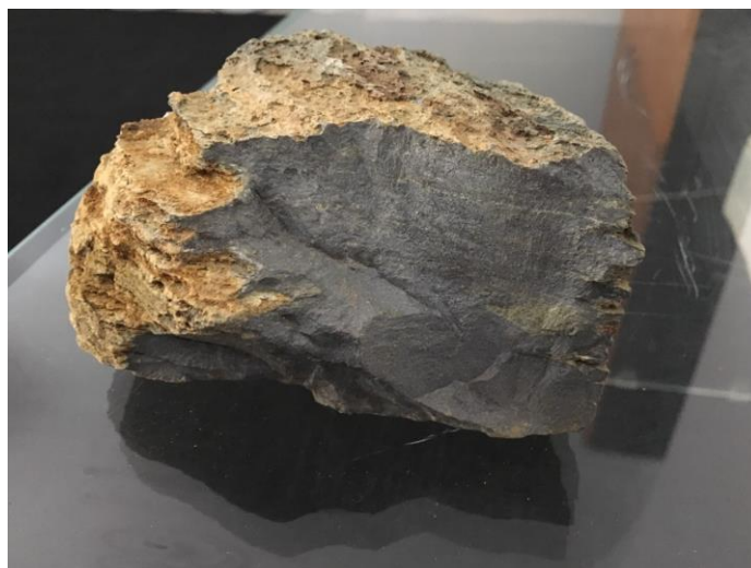
Image 1: Zinc rich massive sulphide rock obtained from Gibson's pit of dimension 14cms (l) x 8cms (d) x 9 cms (h)
