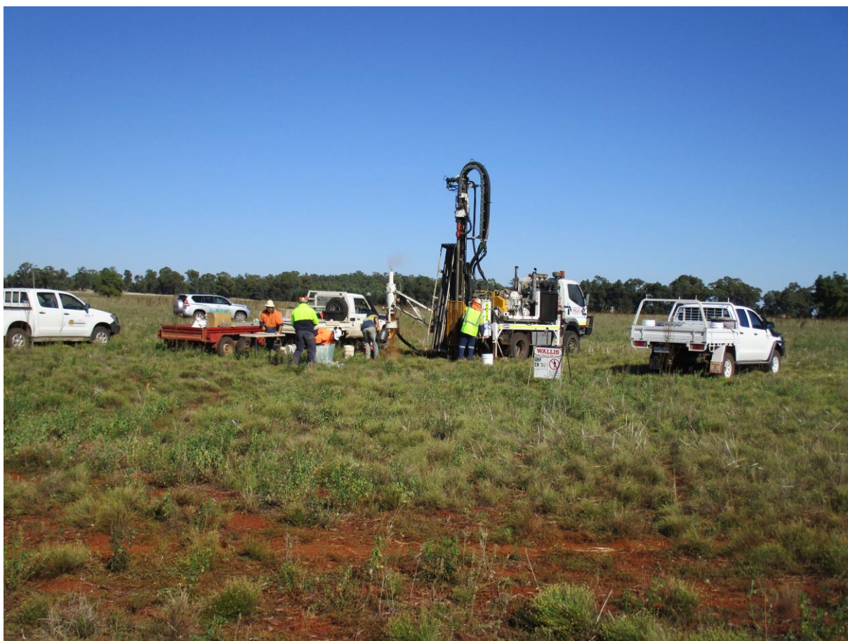
Figure 1: Australian Mines' resource extension drilling at its Flemington Cobalt-Scandium-Nickel Project has commenced. This program comprises 185 air core holes for an expected total of 5,500 metres to be drilled.
