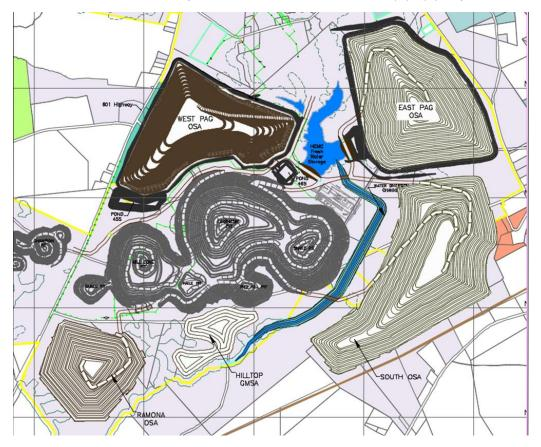
All of the OSAs will be developed with a final reclaimed overall 3(H):1(V) slope.
