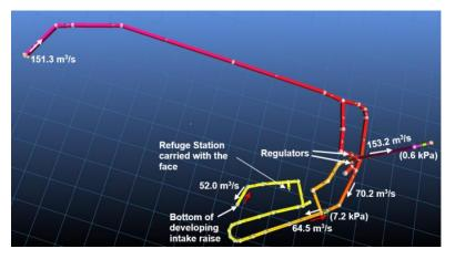
Figure 16-43: Stage 2 airflow distribution
