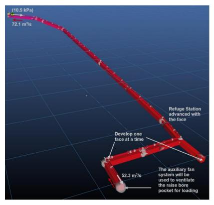
Source: SRK Figure 16-42: Stage 1 airflow distribution
