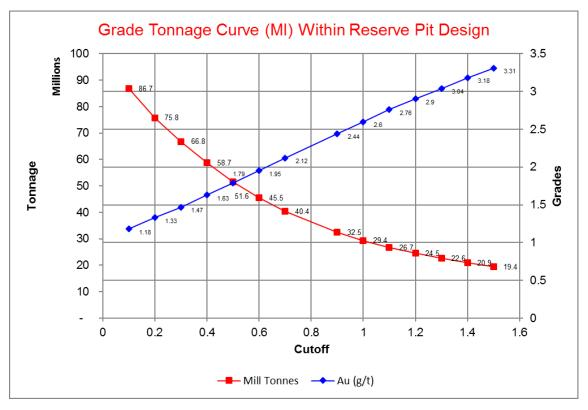
Figure 16-5 shows the grade tonnage curve graphically above a 0.1 g/t lower limit.
