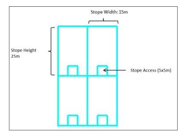
Source: SRK Figure 16-26: Stope Cross Section
