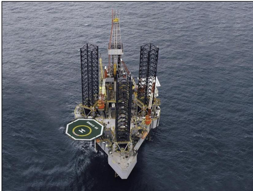
*The Ensco 68 is an independent leg jack-up rig built by Marathon/ Le Tourneau in 1976 and has undergone numerous equipment updates and upgrades since it was placed in to service. Photo courtesy of Ensco Plc.*
