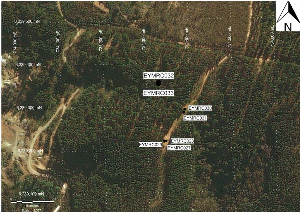
Figure 1: Drill collars of recent RC program (Phase 1 and 2) completed as part of the Lloyds Copper Mine extension program.
