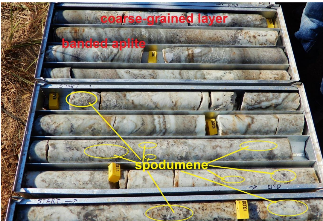
Figure 5: Drill-core attained from MO17DD007, showing layering.
