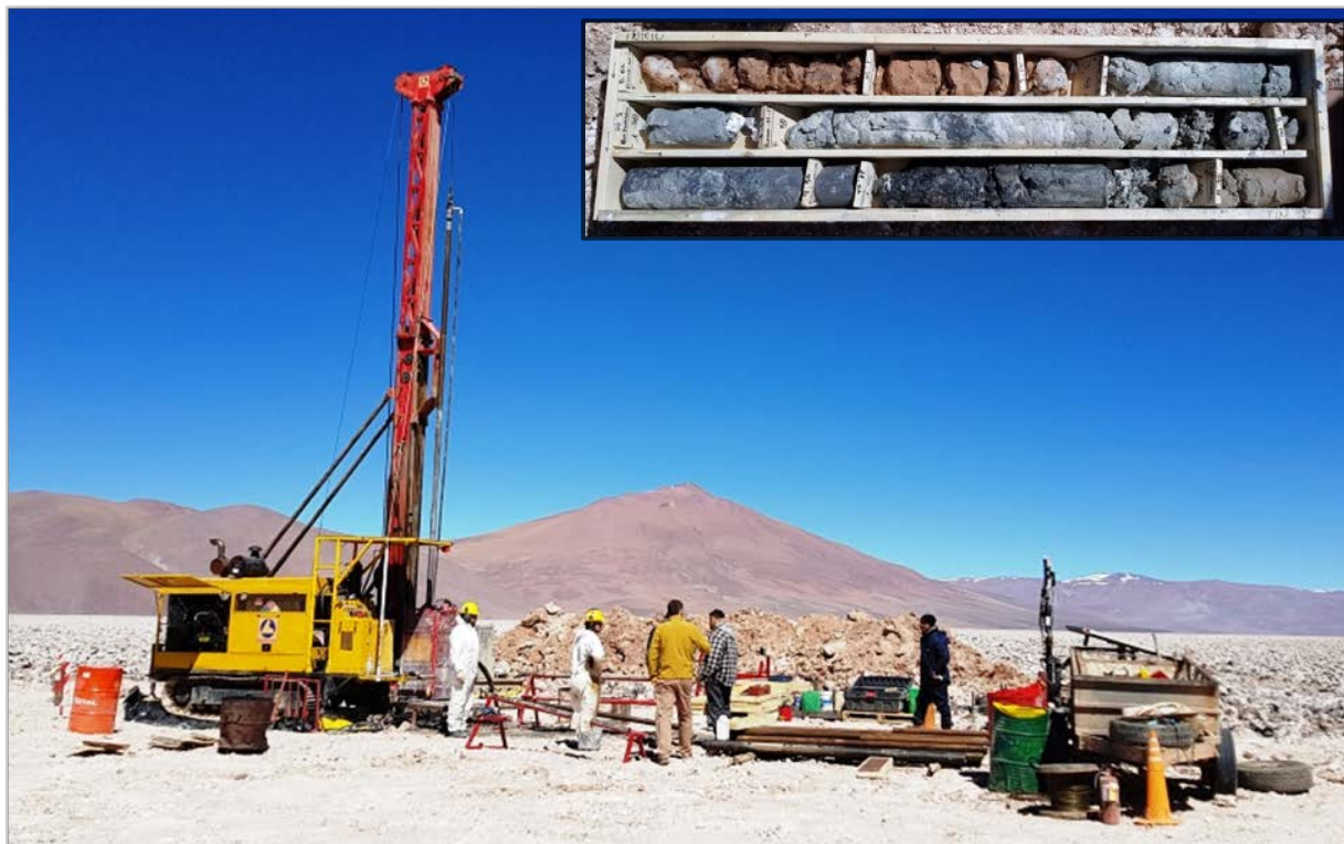
Photo 1. Rincon Lithium Project – Exploration diamond drilling operations and (inset) diamond drill core.
