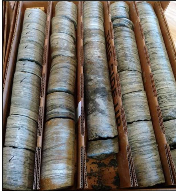
Figure 1: Photo of core from Drill Hole 17FTCBL009 highlighting interbedded colemanite mineralisation.
