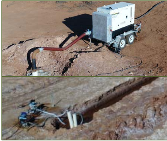
Brine Pumping from Bores and Trenches >80 Million litres successfully pumped to date
