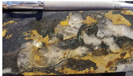
Plate 2. High grade copper mineralisation with coarse quartz (white mineral), biotite-chlorite (dark minerals). Sulphide minerals include chalcopyrite, pyrite and pyrrhotite
