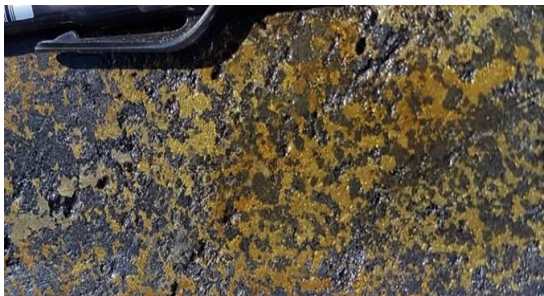
Plate 1. High grade copper mineralisation within magnetite (black mineral). Sulphide minerals include chalcopyrite, pyrite and pyrrhotite.
