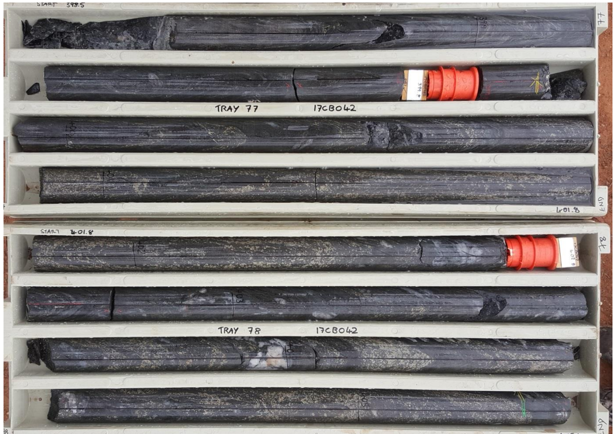
Plate 3. Drill hole from hole 17CB042 (398 to 405 metres) showing cobalt-rich section of core with abundant magnetite (black) and iron sulphide (yellow speckle).
