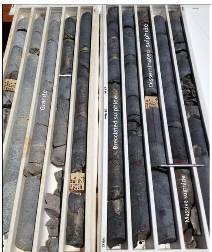
*Figure 3 – core tray from MAD66 showing Ni-Cu sulphide mineralisation*
