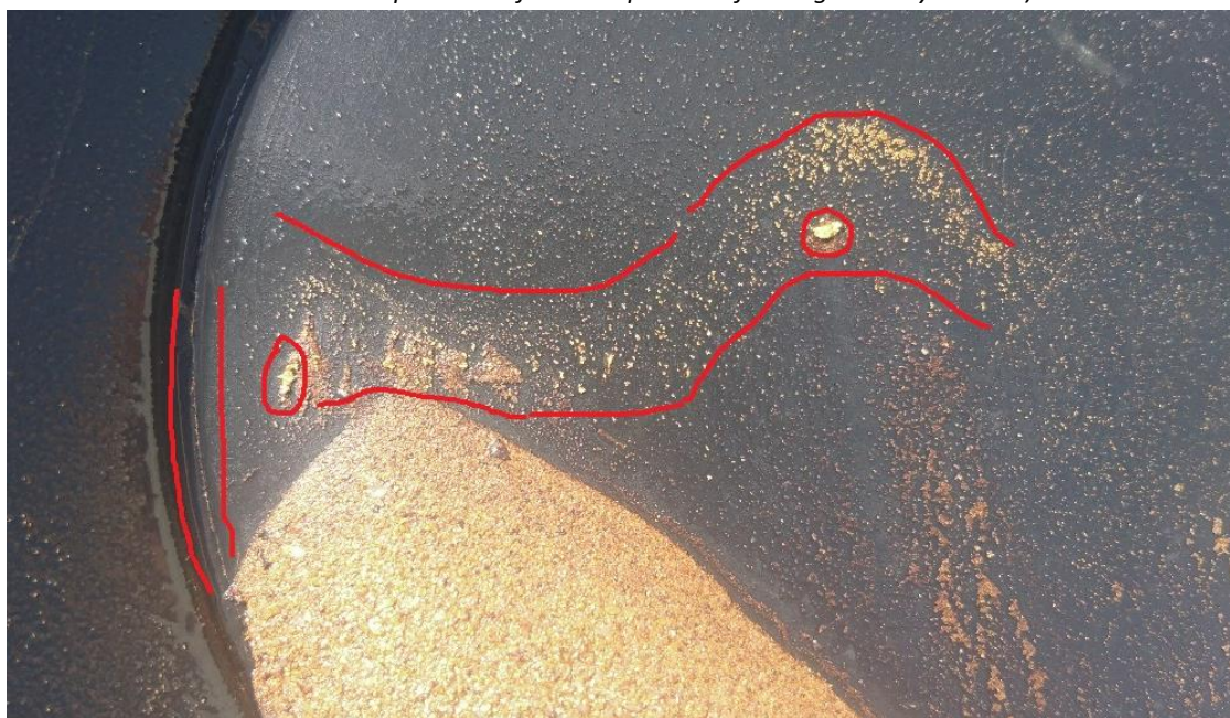
Figure 1: 17RDRC077 7-8m downhole interval, -2mm panned concentrate, fine gold shown inside red bars, larger pieces ~2mm circled
