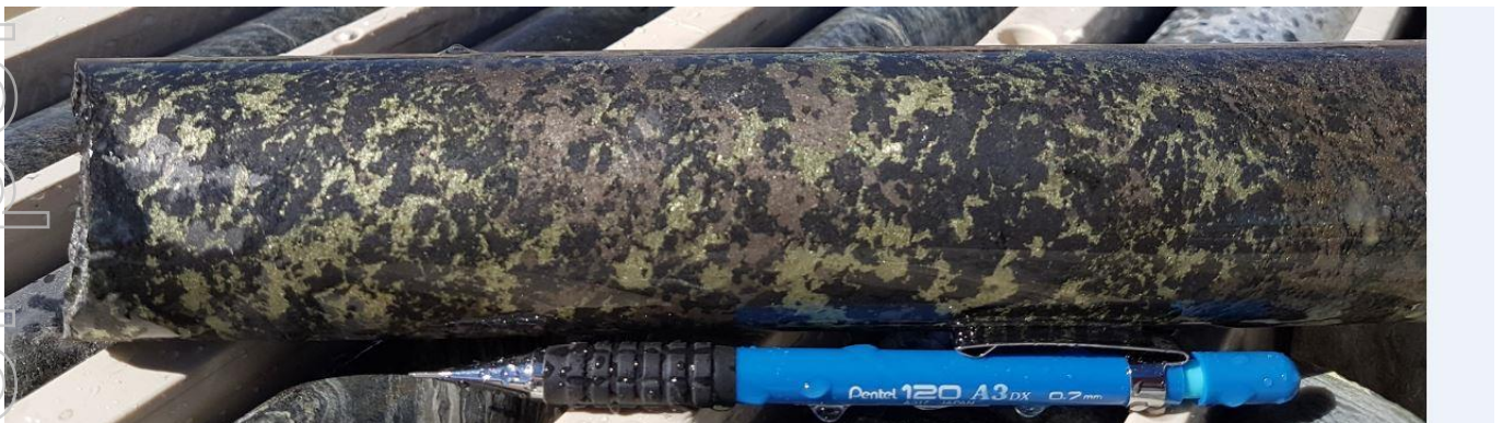
Plate 1 Massive magnetite-chalcopyrite-pyrrhotite-pyrite vein 18CB053. Yellowish mineral is chalcopyrite (copper sulphide).
