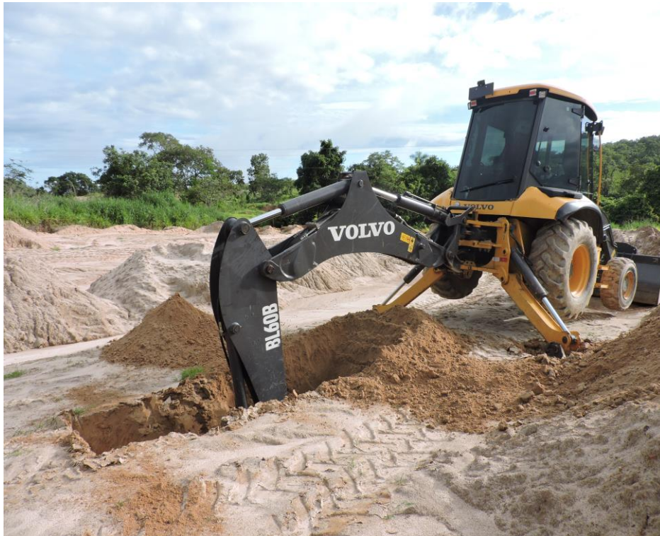
Figure 1; back hoe excavator excavating tailings sample.
