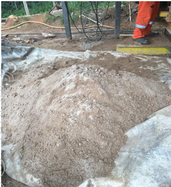
Figures 2 & 3; Samples on Tarpaulin to minimize contamination
