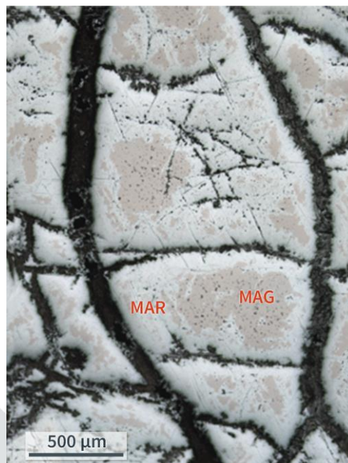
Figure 5 Polished section image of partially oxidised magnetite grain showing a remnant magnetite core and martite (non-magnetic) outer rim.
