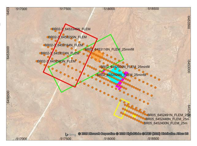
**Figure 2:** Proposed location of Fixed Loop Electromagnetic (FLEM) ground survey stations (shown as orange dots) and transmitter loop (shown as red polygon) compared to the airborne electromagnetic (AEM) anomalies, which are shown as solid magenta and blue polygons (*Priority One* conductors), solid yellow and orange polygons (*Priority Two* conductors) and outlined in green (*Priority Three* conductors).
