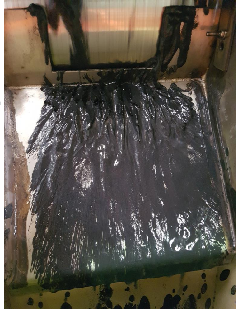
Gabaintha Vanadium Concentrate on pilot scale Low Intensity Magnetic Separation Drum.
