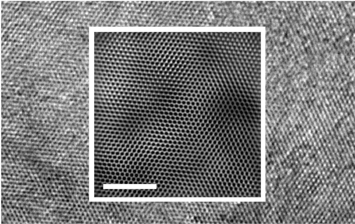
**Fig. 1. An enhanced high-resolution image of Archer's Campoona graphite taken using a JEOL3000F Transmission Electron Microscope showing a highly defined, intricate and periodic honeycomb structure constituting the graphite material. Scale bar represents 2 nm.**
