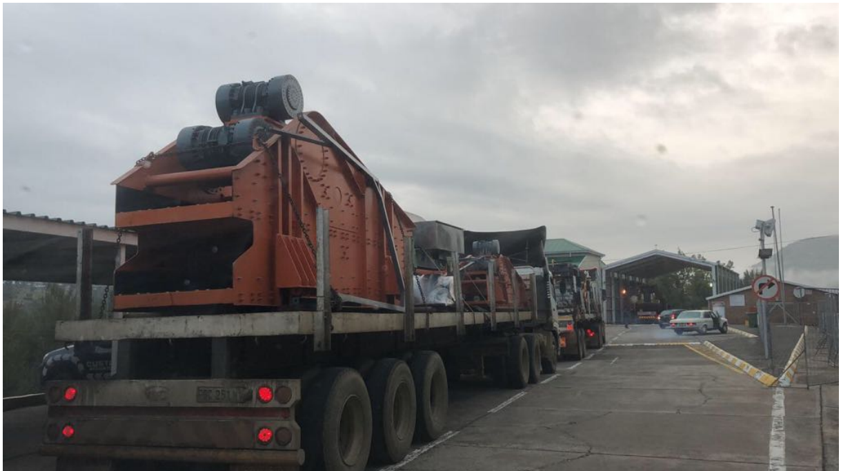
DMS components for the new 150 tph Mothae diamond plant at the Lesotho border
