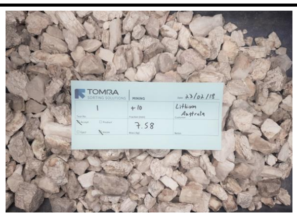
Figure 2: Ore-sorting reject material (mainly feldspar) from Lepidolite Hill mine dumps.
