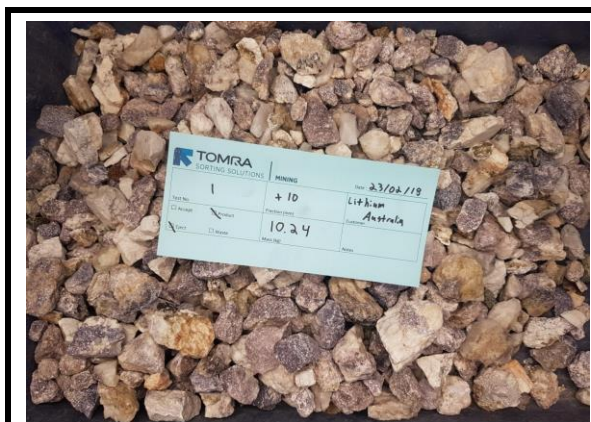
Figure 1: Ore-sorting beneficiated product from Lepidolite Hill mine dumps.
