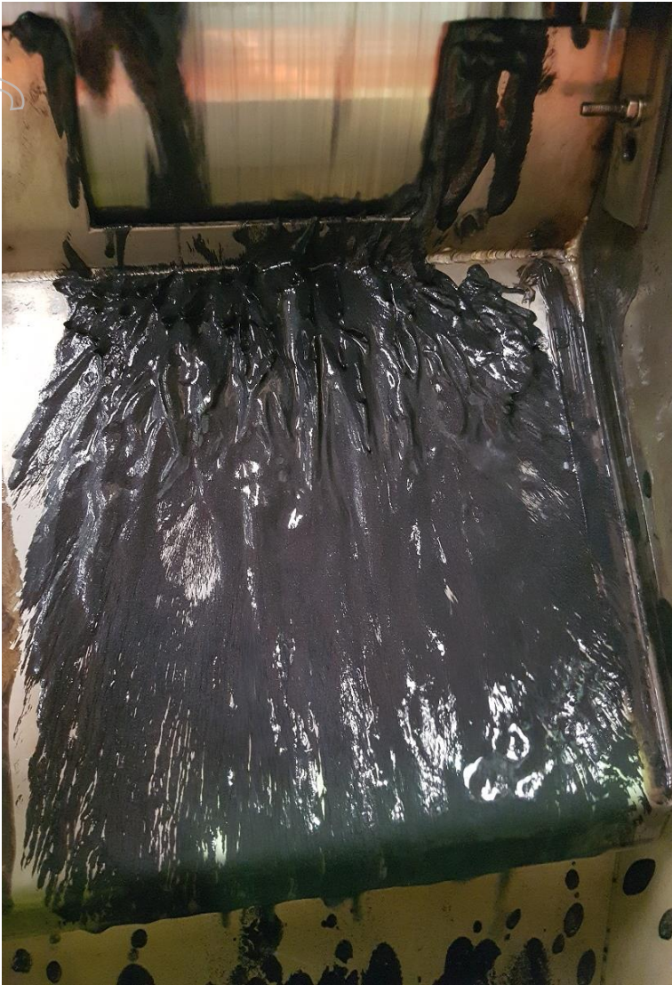
Figure 1: An example of magnetic concentrate (titaniferous magnetite containing vanadium) from a fresh rock sample
