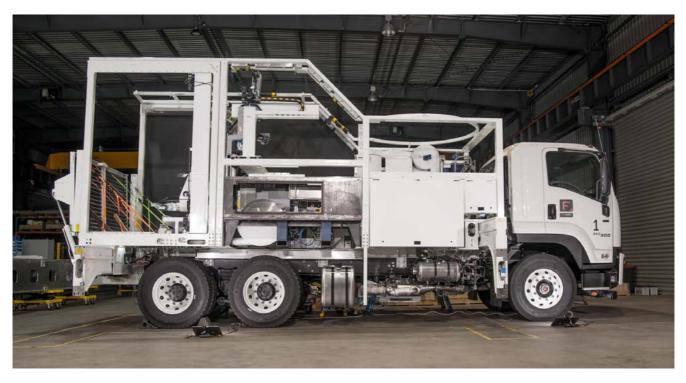
Once the Hadrian X is fully assembled, FBR will then commence testing of the Dynamic Stabilisation Technology (DST) to confirm that the DST meets the functional and technical requirements for the Hadrian X, before entering the Factory Acceptance Testing (FAT) phase, where the Hadrian X will begin to build structures within a controlled factory environment.
