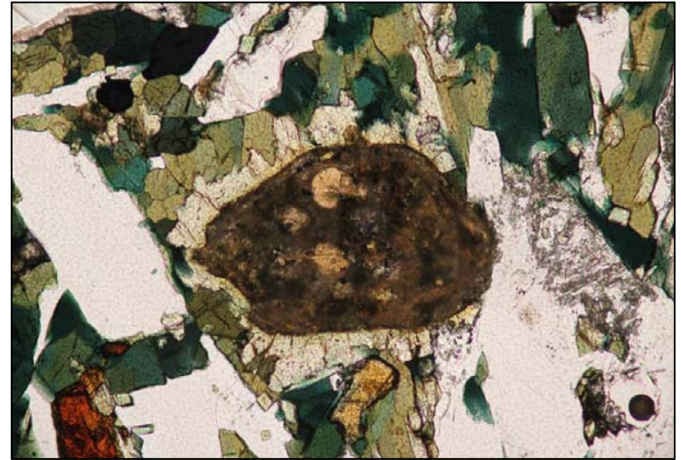
Photomicrograph – steenstrupine grain surrounded by amphibole and feldspar in lujavrite ore
