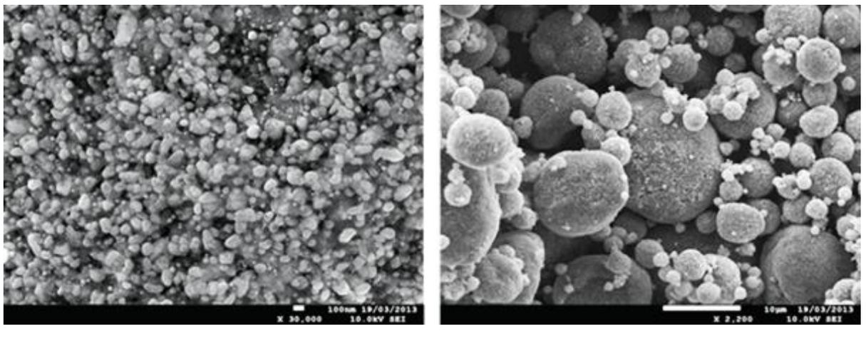
*The image left, above is cathode powder produced using VSPC technology. The scale bar is 100 nanometres (1000 nanometres = 1 micron). The right-hand image shows aggregate VSPC particles (scale bar 10 microns) produced in the typical size range used in LIB cathode powders.*
