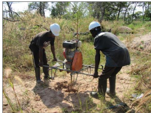
Figures 5 and 6. Power auger drilling testing bedrock geology under cover and in areas of artisanal mining activity
