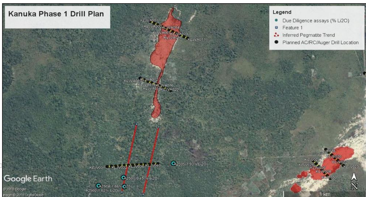
Figure 9. Drill plan for the West Pegmatite with Fences 4, 6 and 7 comprising 13 AC/RC holes to test strike continuity south near previously reported high grade lithium assays and 20 auger holes testing the West Pegmatite
