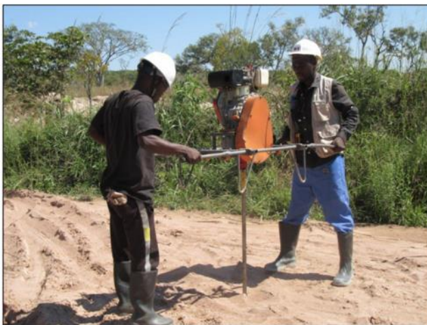
Figures 5 and 6. Power auger drilling testing bedrock geology under cover and in areas of artisanal mining activity
