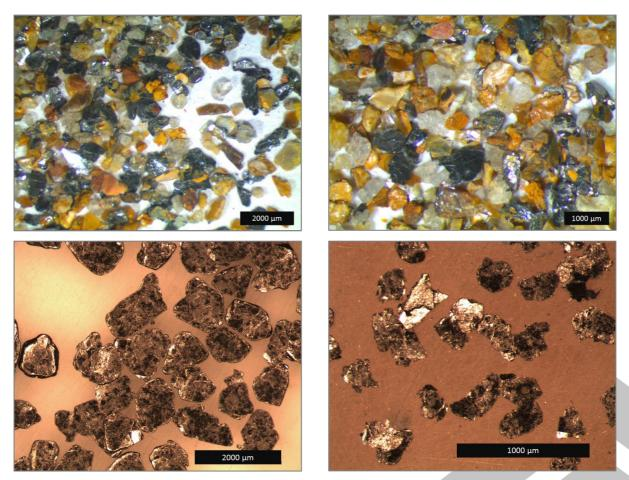
Figure 1: Images of +300µm fraction of scrubber product from Master Composite (top L) and Saprock (top R) showing well liberated graphite flakes amongst quartz-dominant gangue. +500µm super-jumbo flake final concentrate (bottom L) and +150µm medium flake final concentrate (bottom R).
