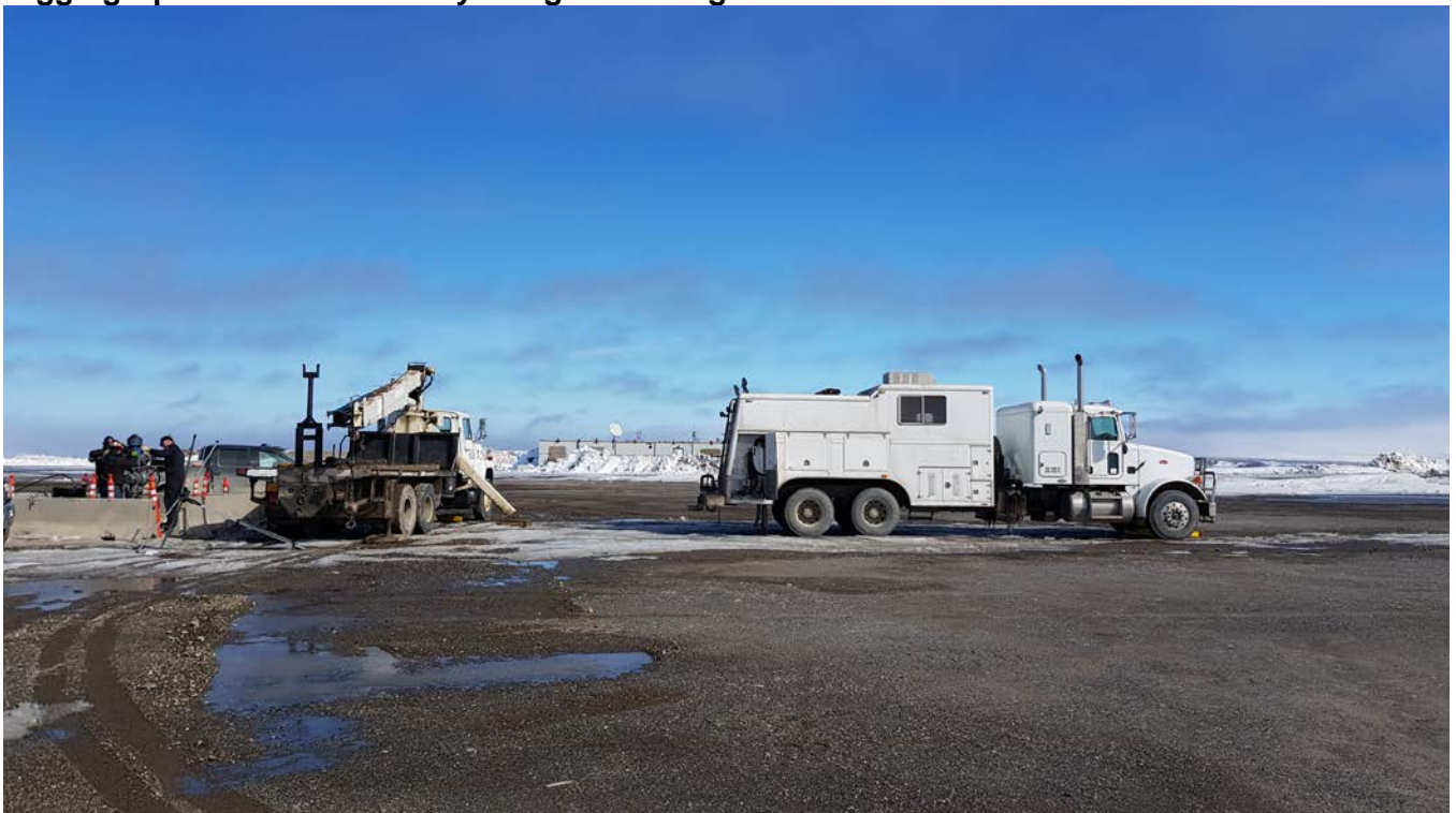
Rigging Up to Retrieve Memory Gauges and Tag Bottom
