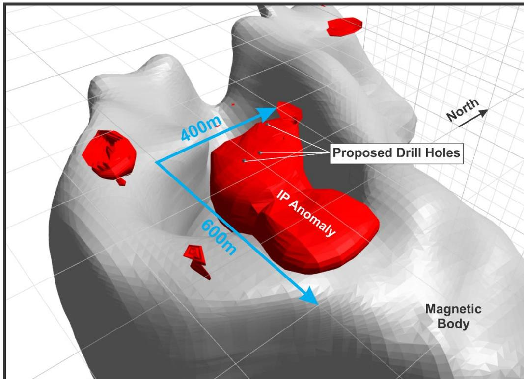
**Figure 2: 3D Chargeable IP Anomalies with Drill Targets**
